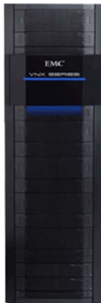
Figure 3-17. EMC VNX 5500 Storage Array.
