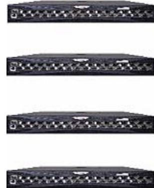
Figure 1.6. 4 Brocade fiber channel switches provide the connectivity for the servers that access the SAN and the tape libraries shown above.
